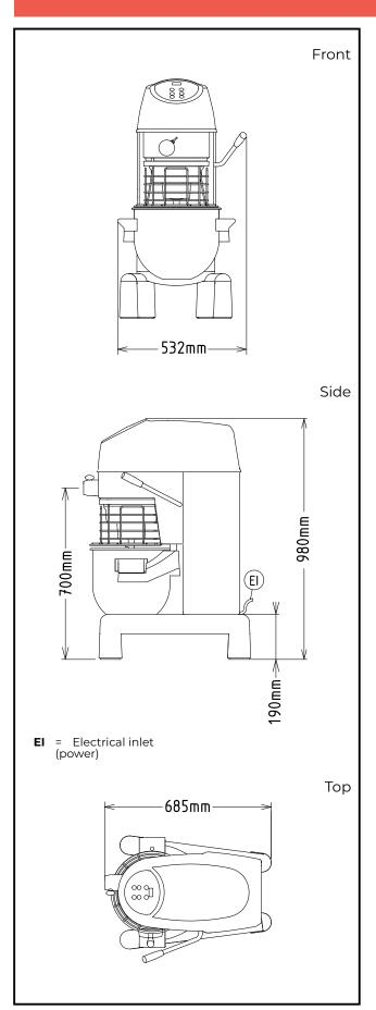
Electric Supply voltage: 200-240 V/1N ph/50/60 Hz **Electrical power max:** 1.01 kW **Total Watts:** 1.01 kW Capacity: Performance (up to): 6 kg/Cycle Capacity: 20 litres Key Information: External dimensions, Width: 521 mm External dimensions, 685 mm Depth: External dimensions, Height: 980 mm ISO 9001; ISO 14001; ISO **Shipping weight:** 45001; ISO 50001 kg Net weight (kg): **Cold water paste:** 6 kg with Spiral hook
